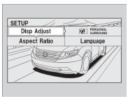
Press the **SETUP** button while the DVD is playing to see the available options. Use the  $\triangle$ ,  $\bigvee$ ,  $\triangleright$ , and  $\triangleleft$  buttons to highlight the option and then press the **ENTER** button.
