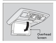
Pull down the screen to the first or second detent until it latches
