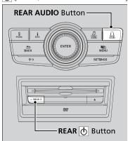
■ REAR AUDIO button on the front panel When you press the REAR AUDIO button, the front display changes to what is displayed on the rear overhead screen.
